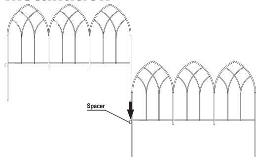
Identify the flush side and spacer on each fence panel.
