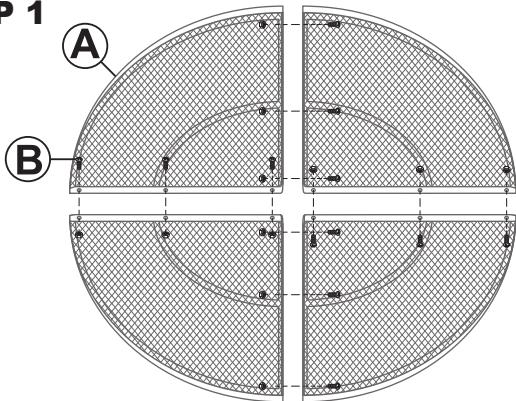
Loosely secure Screen Panels (A) by hand-tightening M6x12mm Bolt Sets (B).
